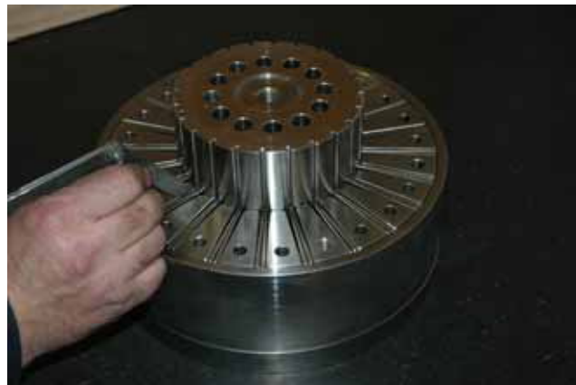
Determining spring preloads during overhaul of small camshaft damper.
